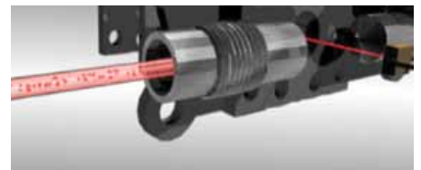
Fig 1. In simple terms a controlled column of contaminated fluid enters the laser optical scanner chamber. This design maintains contamination distribution within the fluid.
